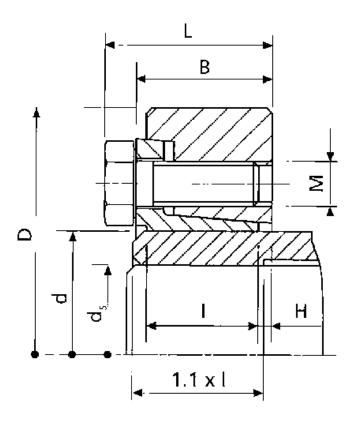
B mm = 31.0 d H8 mm = 80 D mm ds mm = 60 F kN torque = 143
